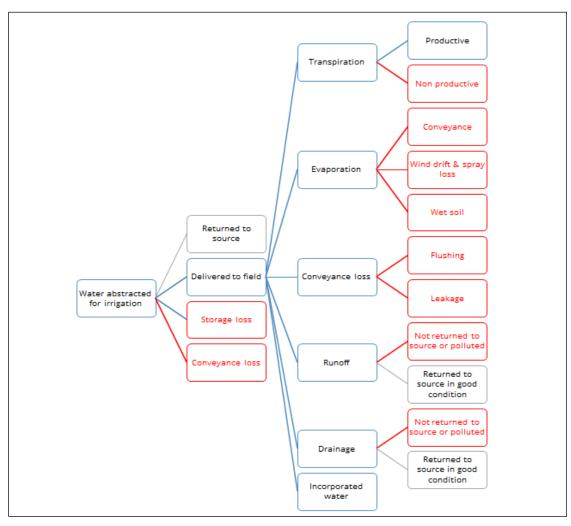
Figure 3 Scheme of Water Use and Water Losses, adapted from BIO Intelligence Service (2012, p. 43)
